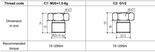
Note: Torque depends on various factors such as material of gasket, supporting materials, lubrication of thread and pressure.
