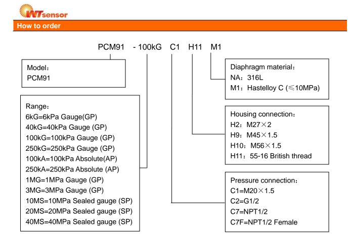
Example: PCM91-100kC1H11 refers to product model PCM91, range  $\pm$ 100kPa Gauge pressure, output: 4 ~ 20mA@HART protocol, pressure port M20\*1.5, housing connection 55-16 British thread and diaphragm 316L.
