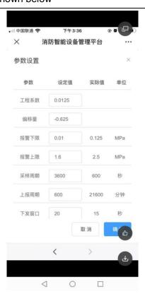
Parameters configured through the platform include: lower limit of alarm pressure, upper limit of alarm pressure, sampling period, reporting period, issuance window, etc.
