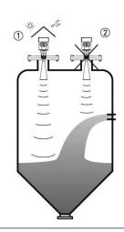
The top conical tank level, can be installed at the top of the tank is intermediate, can guarantee the measurement to the conical bottom.
