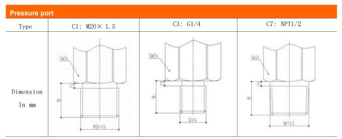
Note: Common threads are M20×1.5, G1/4, G1/2, M14×1.5, NPT1/4 and NPT1/2. Special threads can be customized for batch order.
